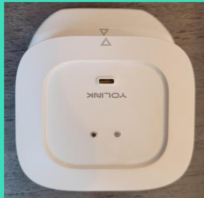
The device has an arrow on one side of the top. The base also has an arrow on the top of it. These arrows must be aligned
